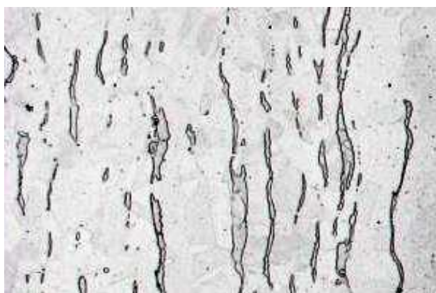
1.4306 untreated steel Austenite and 5% ferrite delta
