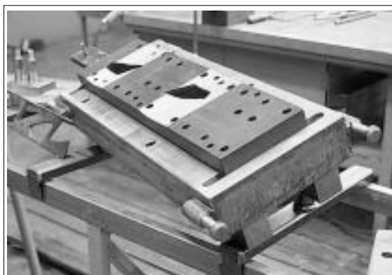
Blanking tool set for producing a plate part.
