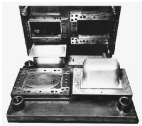
Clipping and edging tool in AISI O1 tool steel to clip and form edge of 0.036" (0.914 mm) thick stainless steel container approx. 10" x 6" x 8" (254 x 152 x 203 mm).
