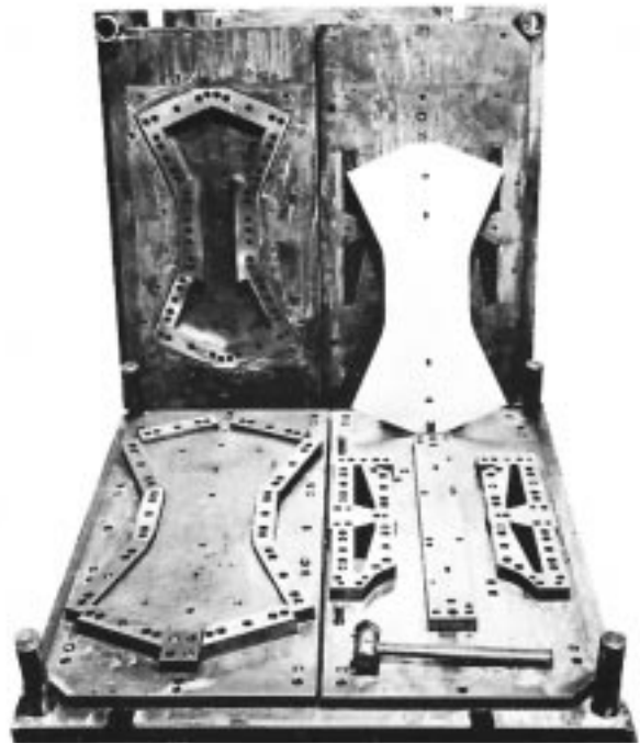
Blanking tool made from fine-machined AISI O1 tool steel.
