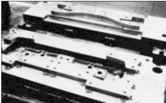
Typical blanking die where CALMAX could be used because of the high demands on toughness.
